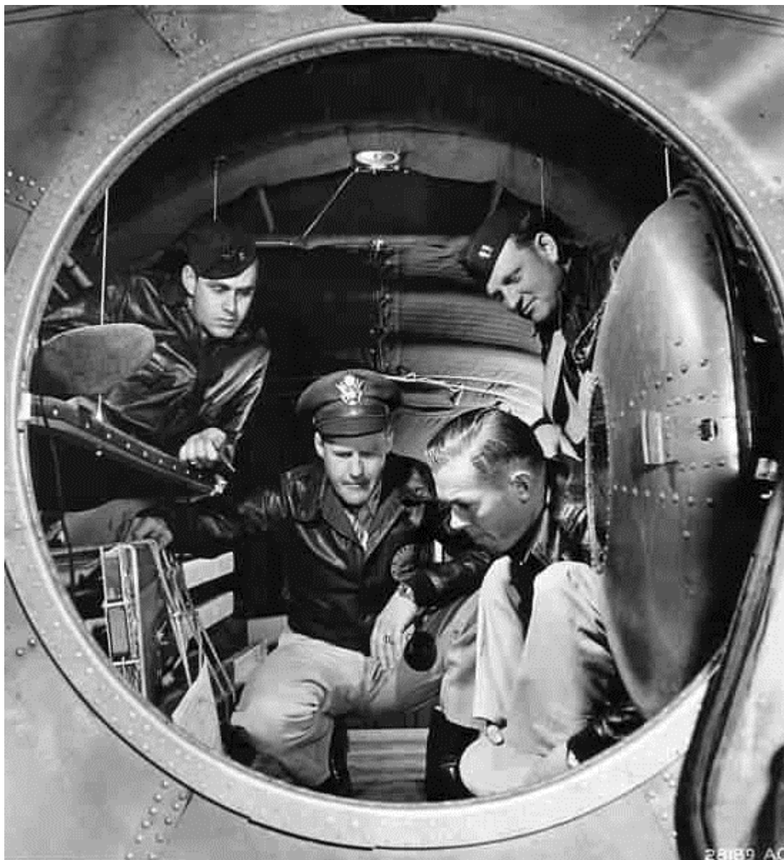
B-29 Super-fortress Rear Pressurized Hull (Crew Rest, 4 bunks)
