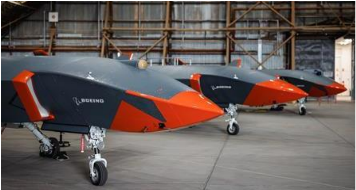
The nose of the MQ-28A is designed to be reconfigurable based on specific missions Source: Commonwealth of Australia
