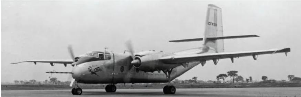
The first Caribou prototype, CF-KTK-X, seen here with a nose probe, made its maiden flight on July 30, 1958. It featured the original short fuselage design, which was later extended forward of the wing to better align with the aircraft's center of gravity
