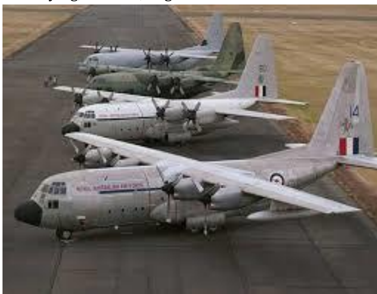
All four models of the Hercules operated by the RAAF. In the foreground is the 'A' model followed by the 'E', the 'H' and the 'J'. I flew the 'A' and the 'H' models.
